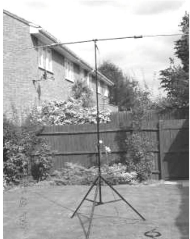
Firstly, I will explain what a Buddipole Aerial is. It is an HF portable dipole aerial system which is designed to be modular, versatile, and effective. It is manufactured by Budd Drummond W3FF in America. The frequency range is from 40m through to 2 m.
