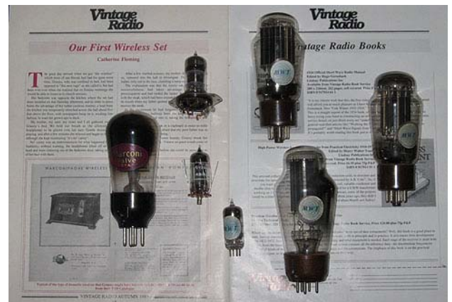
Valves Collection: Left is a Marconi PT2 (Tetrode) from 1925, to the right are the "wired in Valves".
