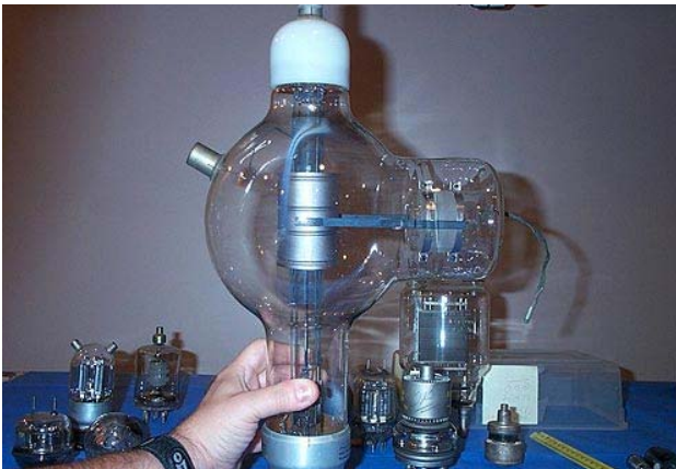
A rare 1938 type JAN861 Tetrode amplifier Valve
