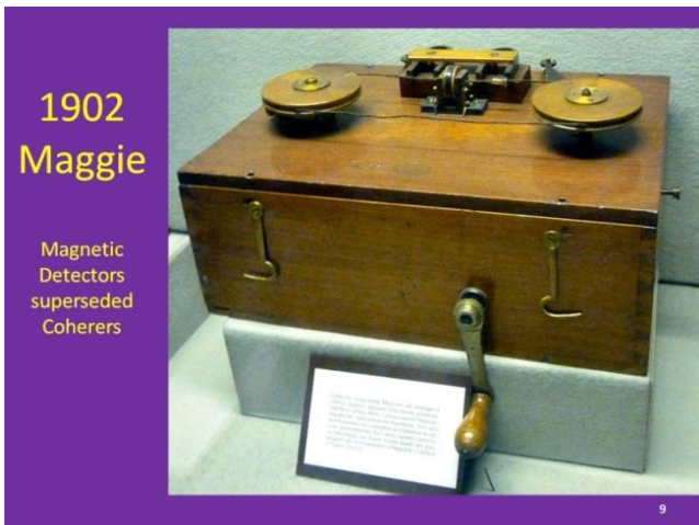
Magnetic detectors (Maggies) were preferred in service to early coherers
