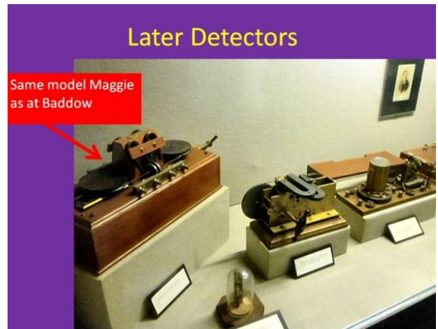
Magnetic detectors (Maggies) were preferred in service to early coherers
