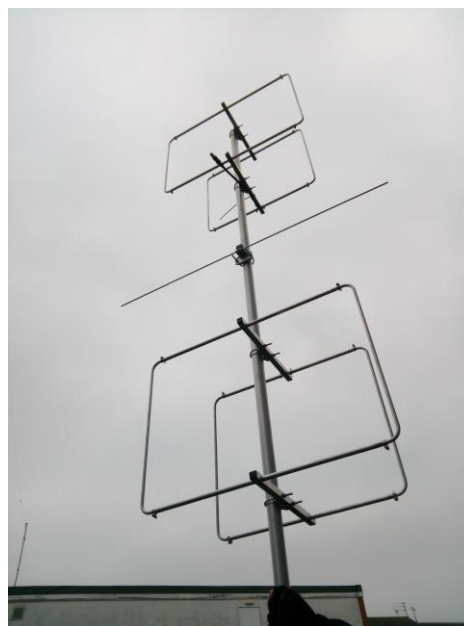
Use of Interleaved parasitic elements between stacked antennas
