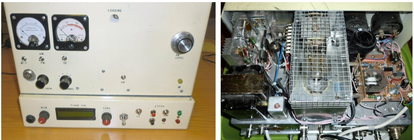
Peter G3SUY: 144 MHz Transceiver Valve PA topside – but with Synthesiser+CTCSS
