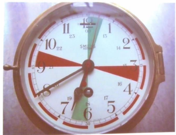
A ships radio room and a clock with the quarter hour emergency watches marked in colour
