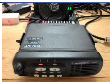
Radio - Motorola GM340 (ex-PMR) with extra cooling fan
