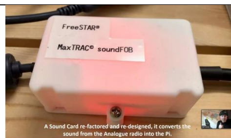
Soundcard to convert the radio analogue sound into the RasPi
