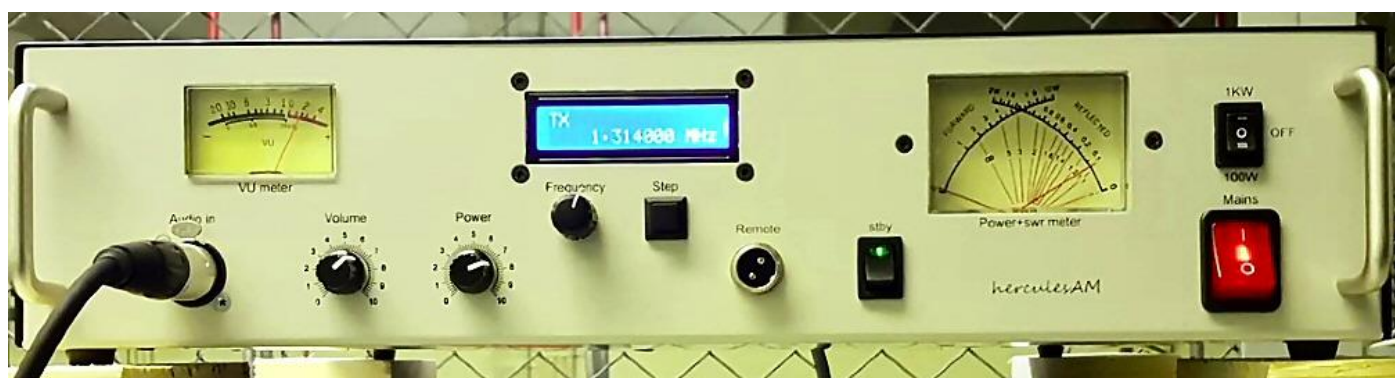
The modern MW transmitter with a 1kW Class-E PA is rather more compact and efficient!
