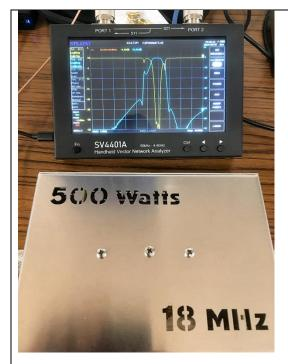
CARS HF 18MHz Bandpass Filter being measured on a SV4401 Vector Network Analyser over 1-30MHz.
