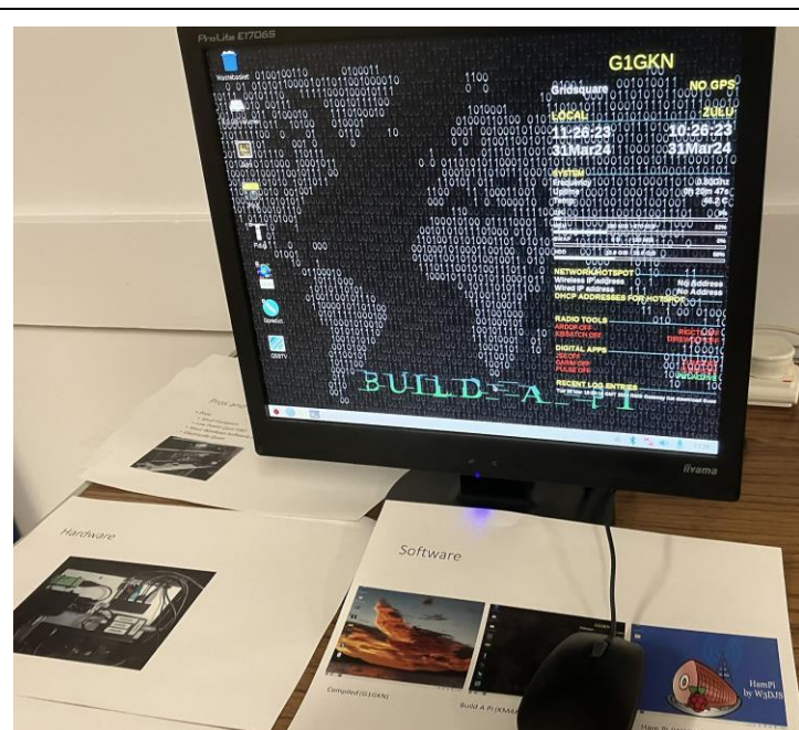
Integrated Monitor, Sound, Raspberry-Pi and RTL Dongle (all attached at the rear) – by Andy Tyler G1GKN
