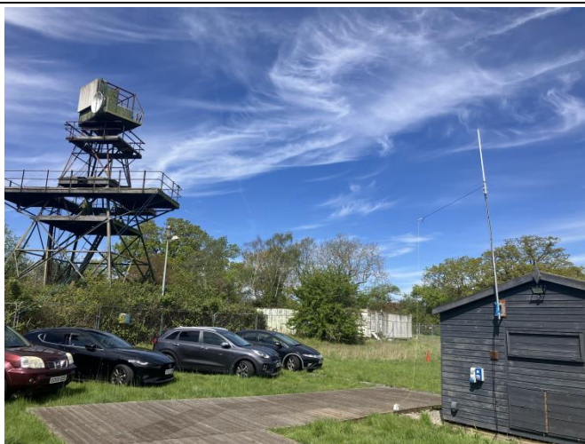
The operating hut in the foreground had an EFHW for HF and Diamond X30. The far end of the EFHW was held up by the Chain Home Low tower
